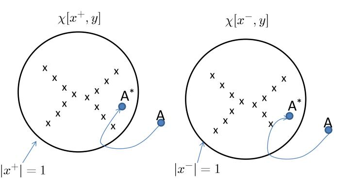
The function  $\chi[x,y]$  may have branch points inside the unit circle. Therefore the analytic continuation via the contour AA<sup>\*</sup> may bring  $\chi[x^+,y]$  and  $\chi[x^-,y]$  (and it does actually) to different sheets. Dealing with the functions on the different sheets is not easy.
